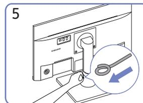
You can remove the fixing pin and adjust the stand now.
