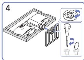
Insert the stand base into the stand in the direction of the arrow. Fasten the screw tightly (using a screwdriver or coin) into the bottom of the stand base.
