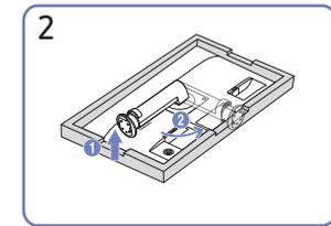
Push the stand neck into the main body in the direction of the arrow as shown in the figure. Tightly fasten the connecting screw on the bottom of the stand.
