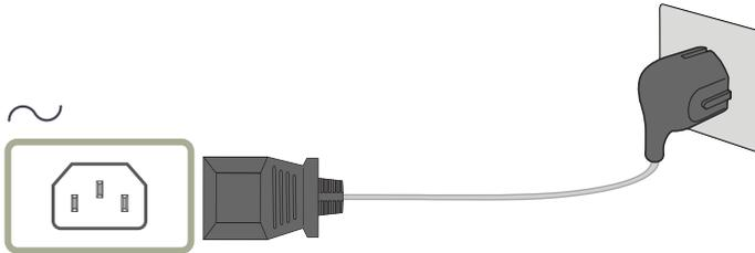
To use the product, connect the power cable to a power outlet and the
