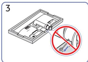
Do not remove the fixing pin until you are finished attaching the stand.
