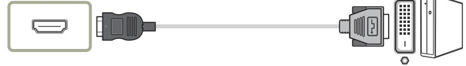
— When using HDMI-DVI cable, audio may not be supported according to source device.
