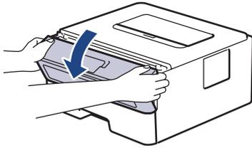
2. Remove the toner cartridge and drum unit assembly from the machine.
