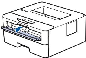
3. Use both hands to slide the manual feed slot paper guides to fit the width of the paper you are using.
