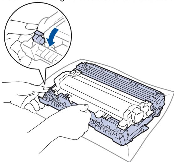
7. Turn the drum unit as shown in the illustration. Make sure that the drum unit gear (1) is on the left side.
