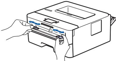
4. Using both hands, place one sheet of paper in the manual feed slot until the front edge touches the paper feed roller. When you feel the machine pull it in, let go.
