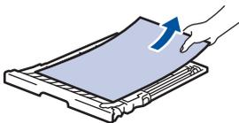
5. Remove paper that may have jammed under the machine due to static electricity.
