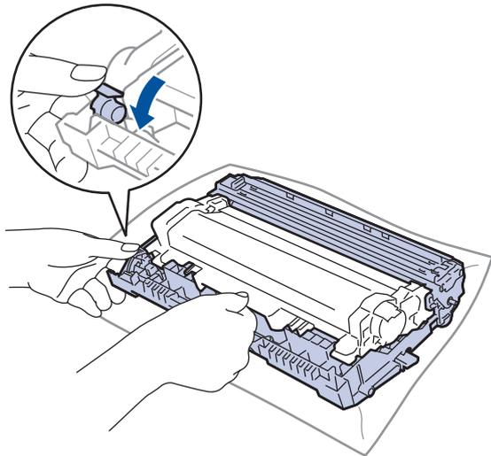
10. Turn the drum unit as shown in the illustration. Make sure that the drum unit gear (1) is on the left side.
