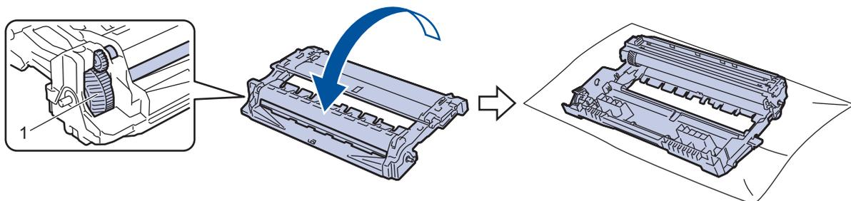
12. Push the toner cartridge firmly into the drum unit until it locks into place.
