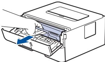
9. Push down the green lock lever and take the toner cartridge out of the drum unit.
