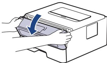
5. Remove the toner cartridge and drum unit assembly from the machine.
