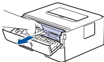
6. Push down the green lock lever and take the toner cartridge out of the drum unit.
