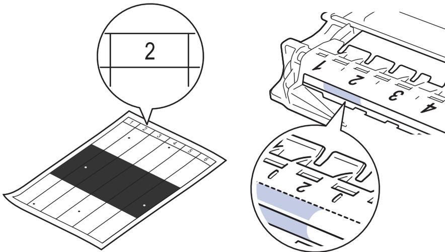
12. Turn the drum unit edge towards you while looking at the drum surface to find the mark.
