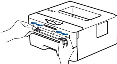
4. Using both hands, place one sheet of paper in the manual feed slot until the front edge touches the paper feed roller. When you feel the machine pull it in, let go.
