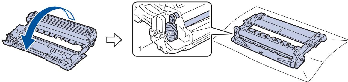
11. Use the numbered markers next to the drum roller to find the mark on the drum. For example, a dot in column 2 on the check sheet means that there is a mark in drum region "2".
