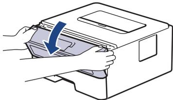
3. Remove the toner cartridge and drum unit assembly from the machine.
