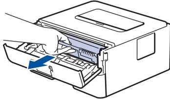
3. Clean the corona wire inside the drum unit by gently sliding the green tab from left to right and right to left several times.
