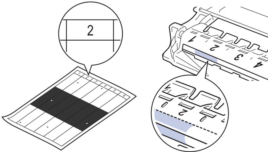
9. Turn the drum unit edge towards you while looking at the drum surface to find the mark.
