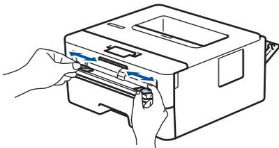
5. Using both hands, put one envelope in the manual feed slot until the front edge touches the paper feed roller. When you feel the machine pull it in, let go.
