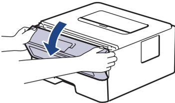
8. Remove the toner cartridge and drum unit assembly from the machine.
