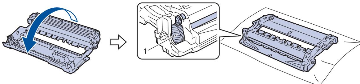
8. Use the numbered markers next to the drum roller to find the mark on the drum. For example, a dot in column 2 on the check sheet means that there is a mark in drum region "2".
