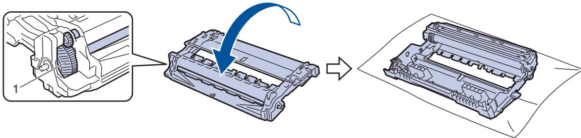
15. Push the toner cartridge firmly into the drum unit until it locks into place.
